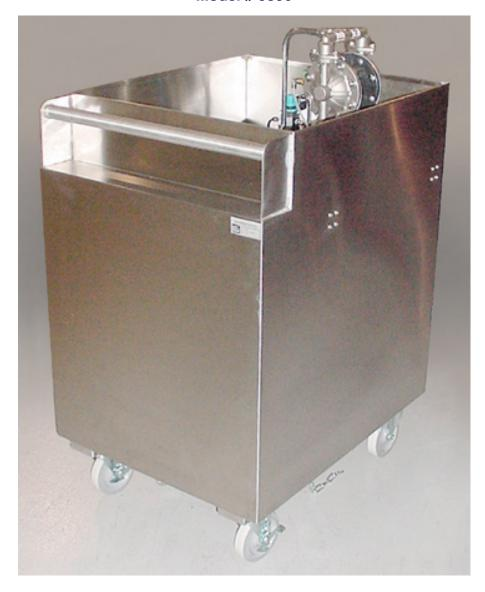
The Solvent Waste Cart is constructed of 304 stainless steel and utilizes a groundable ARO diaphram pump to transfer solvent waste to and from an onboard waste reservoir. It is manually operated with female pipe thread (fpt) connections. It has a footprint of 30" x 24" x 40H" and includes 2 rigid casters and 2 swivel casters with foot brakes. All casters are 5" and nonmar type.
