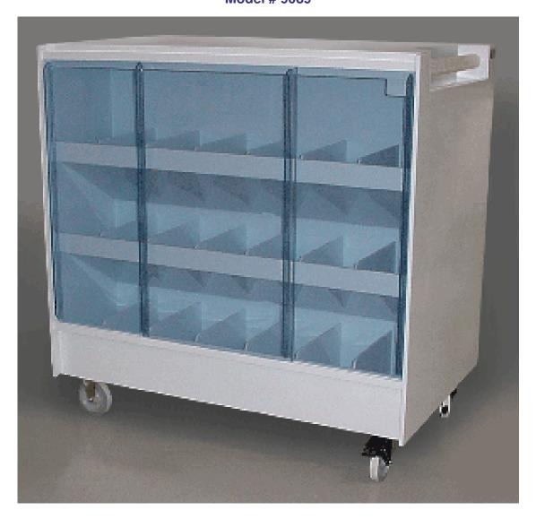
The Acid Bottle Cart is constructed of 1/2" white polypropylene with 1/4" clear PVC sliding bypass doors on either side for ease of access. Each bottle holder is slanted downward and has an open drain to center of the cart for spill containment. A plugged drain port is located at the bottom of the cart. This cart can hold 42, 1-gallon bottles and has a footprint of 48" x 31" x 49H" and includes 2 rigid casters and 2 swivel casters with foot brakes. All casters are 5" and nonmar type.
