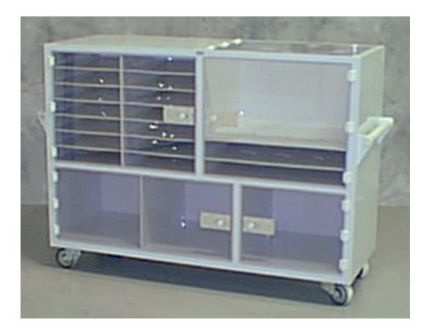
The WIP Cart is constructed of 1/2" white polypropylene and is designed to transport various sizes of product. Hinged, latched doors are made from 1/4" clear PVC doors and this unit has a footprint of 84" x 31" x 63H". Shelving can be designed as removable or fixed. 2 rigid casters and 2 swivel casters with foot brakes are provided. All casters are shock absorbing, 5" and nonmar type.
