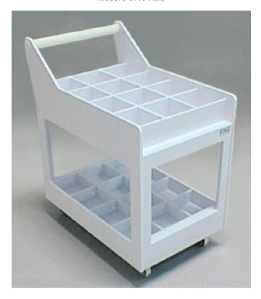
The Acid Bottle Cart is constructed of 1/2" white polypropylene and can hold 24, 1-gallon bottles separated by removable dividers. It has a footprint of 38.5" x 23" x 45H" and includes 2 rigid casters and 2 swivel casters with foot brakes. All casters are 5" and nonmar type.
