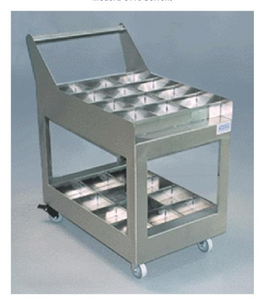
The Solvent Bottle Cart is constructed of 304 stainless steel and can hold 24, 1-gallon bottles separated by removable dividers. It has a footprint of 38.5" x 23" x 45H" and includes 2 rigid casters and 2 swivel casters with foot brakes. All casters are 5" and nonmar type.
