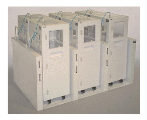
The Transport Carts and Docking Station are constructed of 1/2" white polypropylene with 1/4" clear PVC windows. Each cart measures 32" x 33" x 68"H and is designed to transfer and store parts in a nitrogen atmosphere until needed. All carts come standard with 2 rigid casters and 2 swivel casters with foot brakes. All casters are 3-1/2" and nonmar type.
