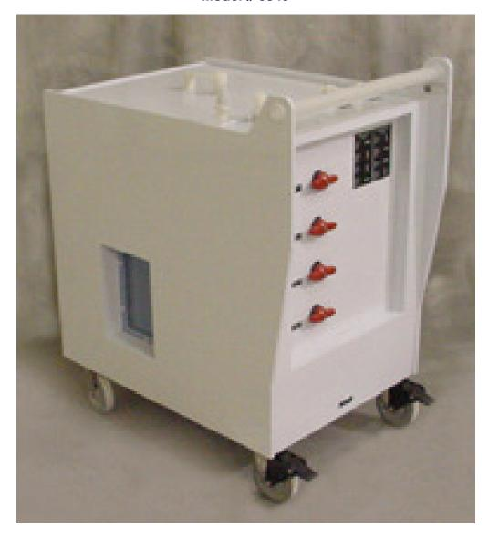
The Chemical Waste Cart is constructed of 1/2" white polypropylene and utilizes an air operated pump to transfer chemical waste to and from an onboard waste reservoir. It is manually operated with guick disconnect inlet and outlet connectors. It has a footprint of 34.5" x 24.5" x 41.5H" and includes 2 rigid casters and 2 swivel casters with foot brakes. All casters are 5" and nonmar type.
