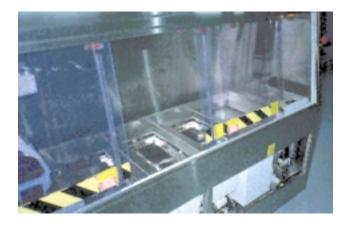
Operator protection features include splash shields of acrylic or PVC, or complete wire glass door assemblies.
