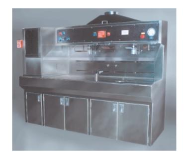
This stainless steel Wax dismounting station is designed for solvent applications. This model features a built-in heated drying chamber with HEPA filtration, and filtered, recirculated solvent dispenser.
