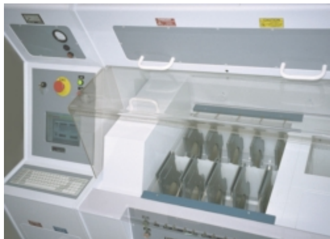
Each plating cell is connected to a separate rectifier, allowing precise plating control.
