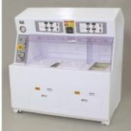
Control panels are mounted beside the work deck, rather than over it. Most wiring and plumbing access is tool-secured, and easily accessible. Safety labeling meets requirements, and components are clearly marked.
