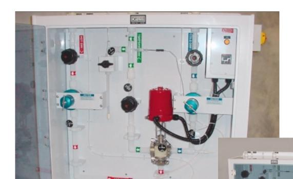
The D.I.W. Blend Station is a freestanding cabinet constructed of 1/2" white polypropylene, with a clear PVC door. This tool is designed to blend hot and cold D.I. water to a specific tool temperature. A 4 to 20ma signal controls blending.
