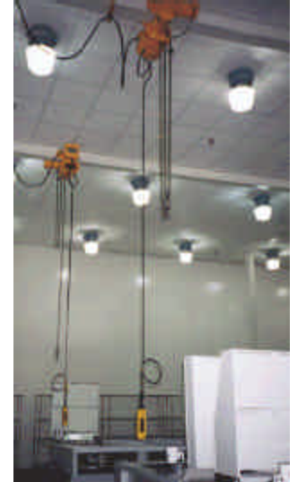
Optional manual (shown) or automated hoist systems are available.
